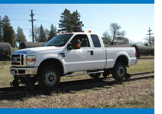
Harsco Rail's LD1515 HY-RAIL® guide wheel equipment is used to adapt light duty trucks and SUV's, meeting Harsco Rail's recommended vehicle specifications, for railway applications requiring travel on the highway and on the rail. Featuring hydraulic locks, push button actuation, electrical track insulation, and mechanical safety pins, the LD1515 has a rugged, compact design that continuously provides the durability needed on the track.
