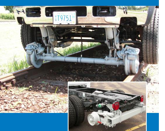
The Harsco Rail MD1920 HY-RAIL® guide wheel equipment is used to adapt medium-duty chassis cab trucks, meeting Harsco Rail's recommended vehicle specifications, for railway applications requiring travel on the highway and on the rail. Featuring hydraulic deployment, hydraulic locks, electrical track insulation, and mechanical safety pins, the MD1920 has a rugged, compact design that continuously provides the durability needed on the track.
