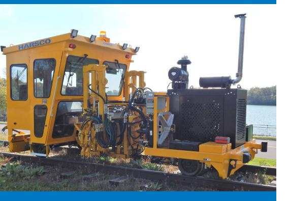
The Harsco Rail SP8A Dual Rail Spike Puller is capable of pulling up to eight spikes simultaneously, even when operating on tracks where both line spikes and anchor spikes are present.
