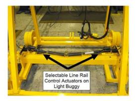
This conversion installs two small actuators that are used to pull the bias spring to the appropriate line rail. A junction box is installed on the light buggy which contains contol relays. One relay is used to supply power to the selected lining light. The other relays are used to control the bias actuators. These relays are controlled using existing on-screen functions.
