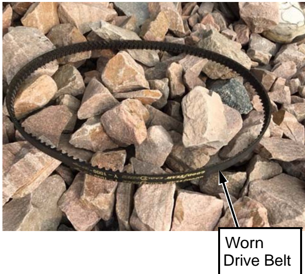
FIGURE 1 WORN DRIVE BELT
