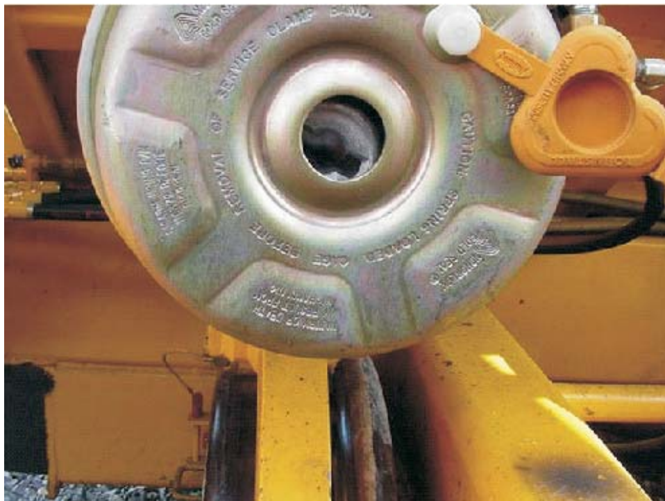
FIGURE 2 MISALIGNMENT OF CAGING SOCKET IN BRAKE CHAMBER
