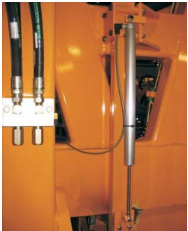
FIGURE 8 NEW TRANSDUCER INSTALLED
