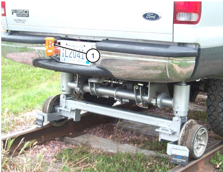
FIGURE 2-1 LOWERING REAR GUIDE WHEELS ELECTRIC LOCK UNIT SHOWN
