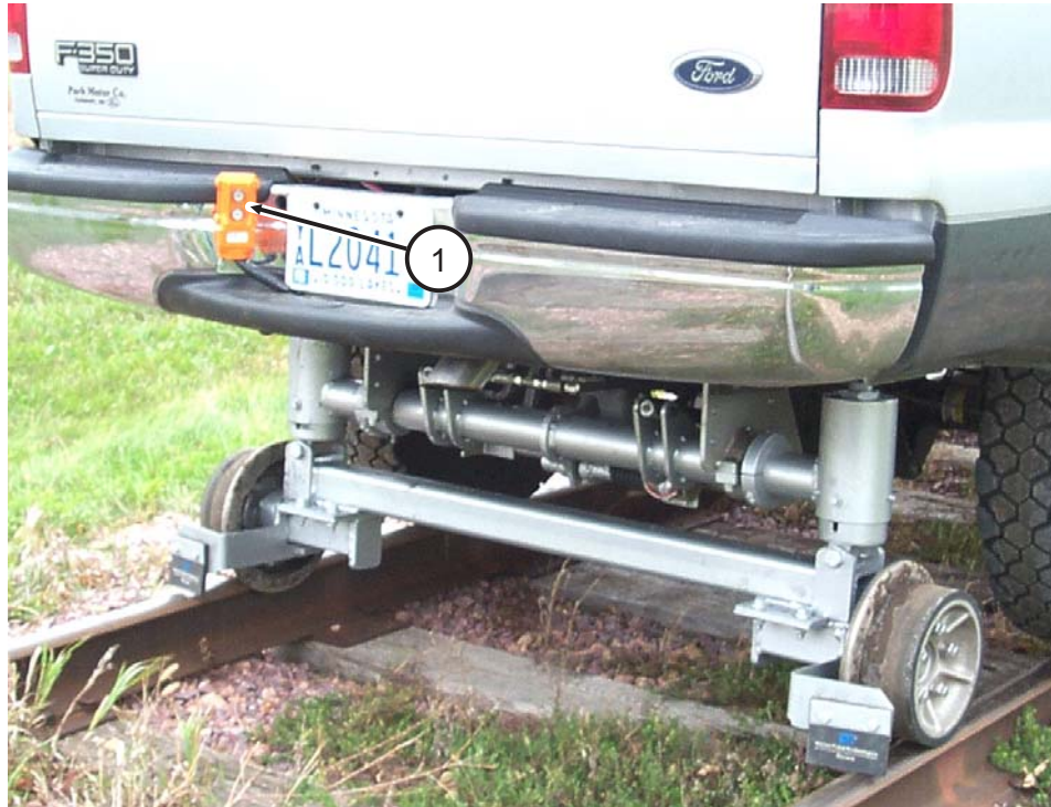
FIGURE 2-15 RAISING REAR GUIDE WHEELS ELECTRIC LOCK UNIT SHOWN
