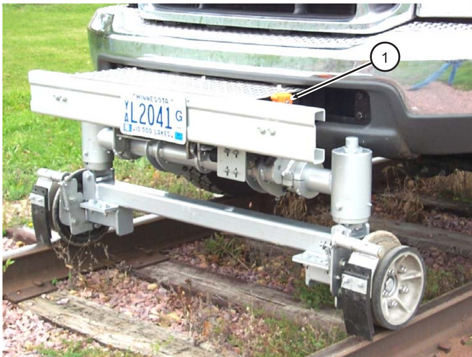
FIGURE 2-4 LOWERING FRONT GUIDE WHEELS ELECTRIC LOCK UNIT SHOWN
