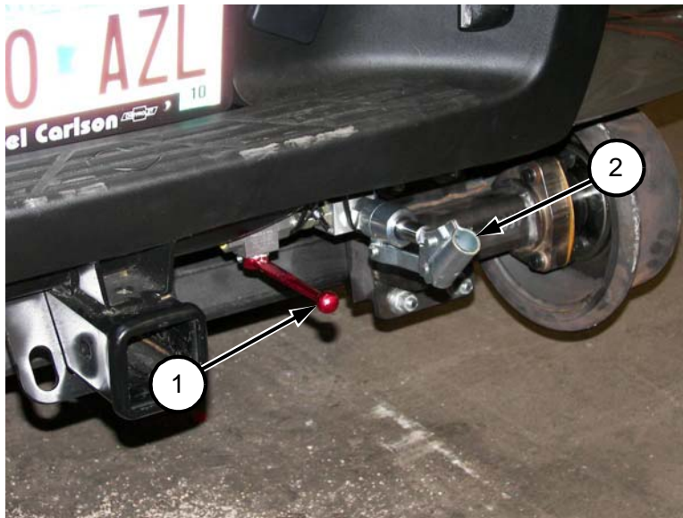
FIGURE 2-14 RAISING GUIDE WHEELS WITH HAND PUMP
