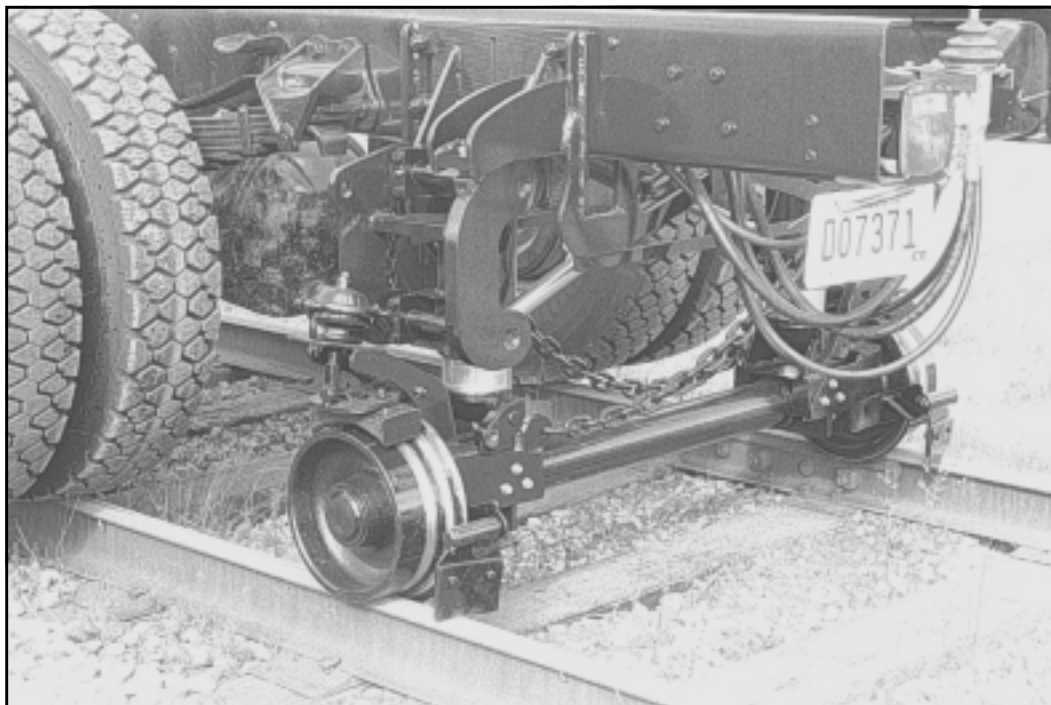
FIGURE 1-1 HR3000 SERIES B REAR HY-RAIL® GUIDE WHEEL UNIT
