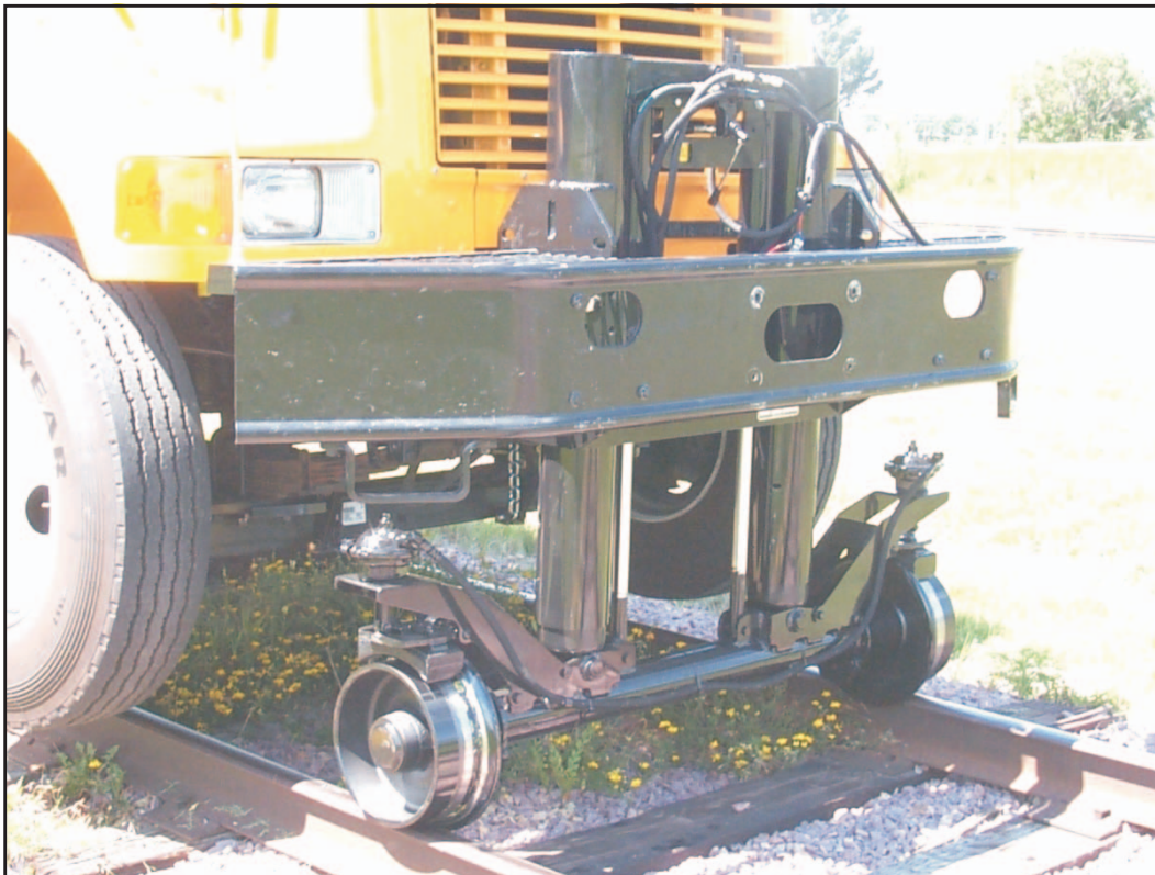
FIGURE 1-1 HR3000 SERIES V FRONT HY-RAIL® GUIDE WHEEL UNIT
