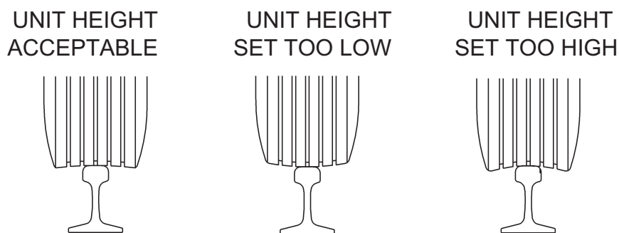
FIGURE 3-4 TIRE PROFILE OVER THE RAIL
