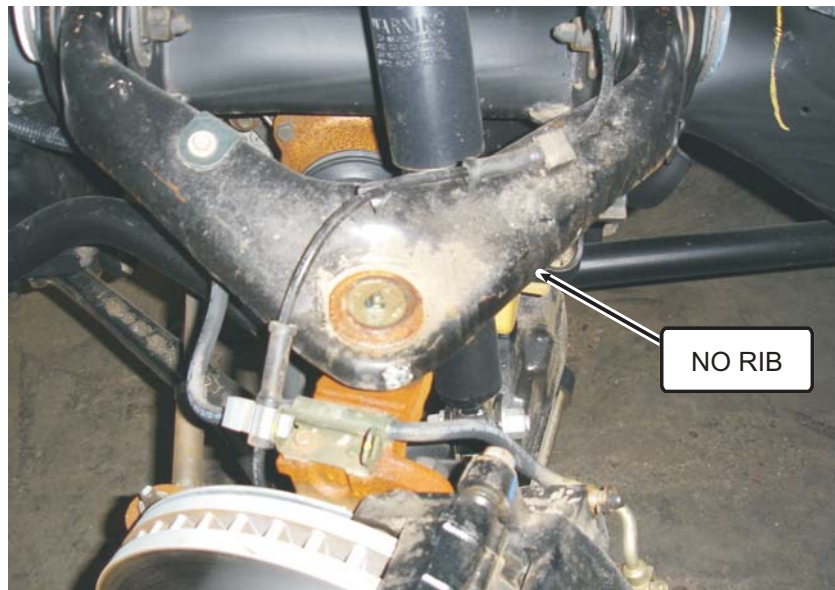
FIGURE 2 UPPER CONTROL ARM WITHOUT RIB
