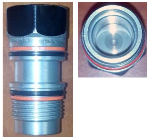
FIGURE 3 CAVITY PLUG - INCORRECT
