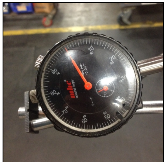
FIGURE 3 HUB ROTATED AND PULLED OUT, INDICATOR READS .020\"/> THIS EXCEEDS 0.005\" SPECIFICATION, INTEGRAL SPINDLE SHOULD BE REPLACED
