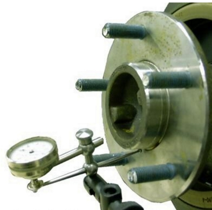
FIGURE 2 HUB ROTATED AND PRESSED IN, INDICATOR ZEROED OUT
