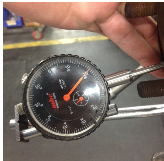
FIGURE 3 HUB ROTATED AND PULLED OUT, INDICATOR READS .020\"/> THIS EXCEEDS 0.005\" SPECIFICATION, INTEGRAL SPINDLE SHOULD BE REPLACED
