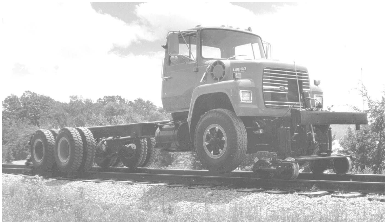
FIGURE 1-1 SERIES 2654 HY-RAIL® GUIDE WHEEL EQUIPPED VEHICLE
