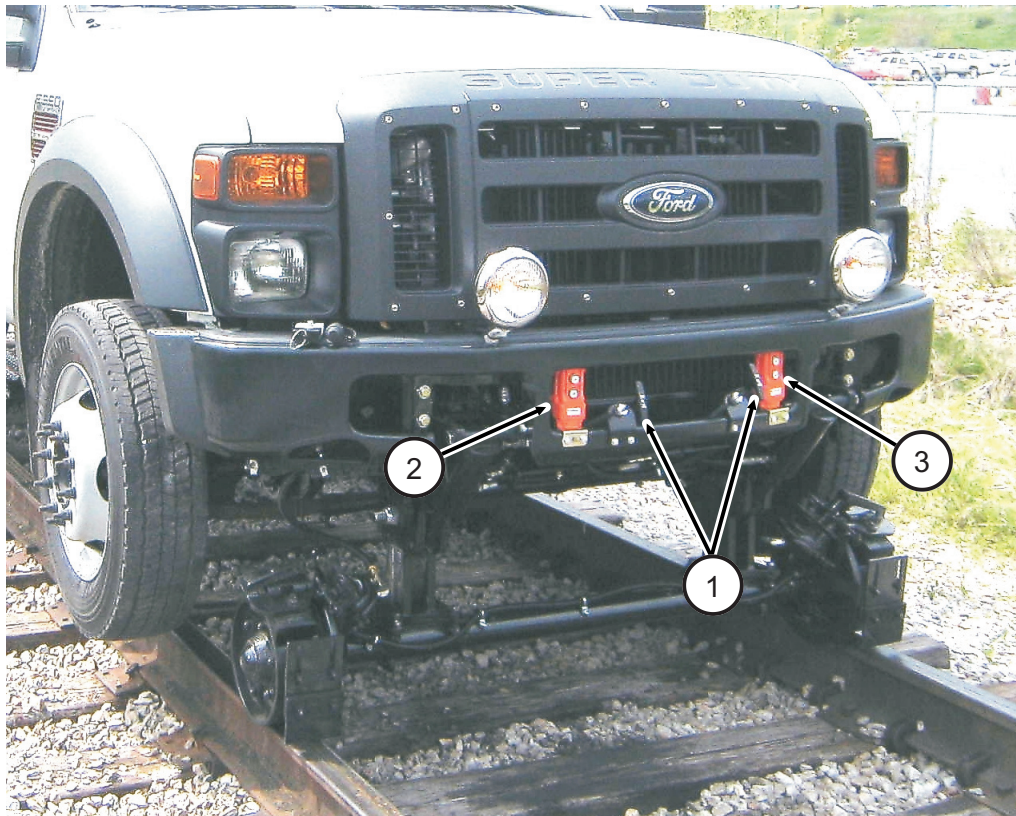
FIGURE 2-1 LOWERING THE FRONT GUIDE WHEELS
