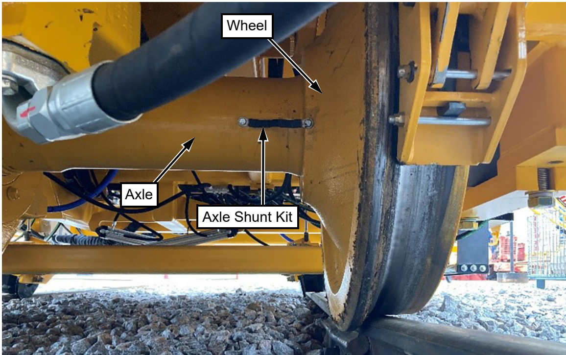
FIGURE 2 AXLE SHUNT KIT INSTALLED
