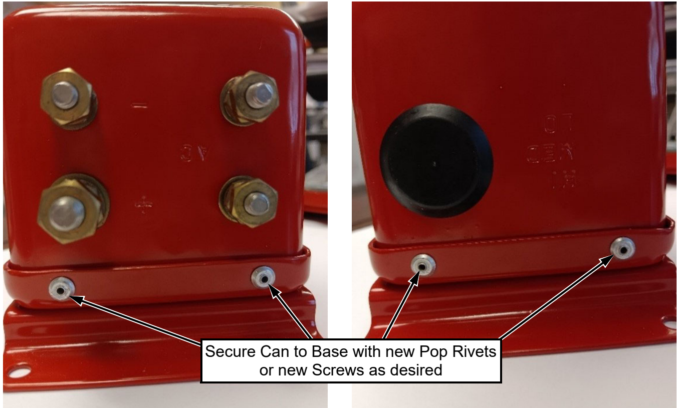
FIGURE 9 SECURING REGULATOR CAN ONTO BASE
